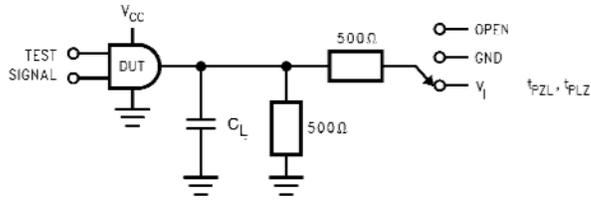
**FIGURE 1. AC Test Circuit (C<sub>L</sub> includes probe and jig capacitance)**
