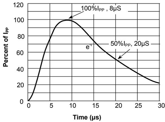
Fig.4 Pulse Waveform-ESD(IEC61000-4-2)
